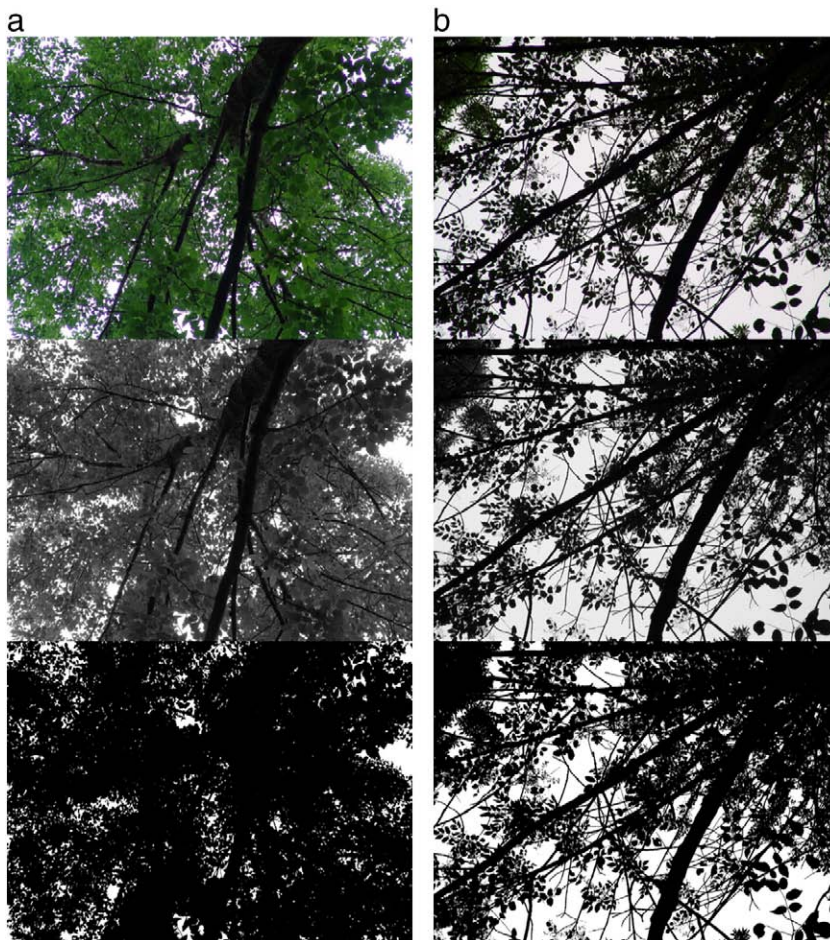
Fig. 2. Digital Canopy Transparency. Percent canopy transparency was quantified using a digital camera zoomed in to four different locations around the canopy. A customized script converts color photographs to grayscale and then to black and white based on a user-defined threshold. Transparency is then calculated as the number of white versus total pixels. The sequence presented here is for a healthy dense canopy (a) and a thinning decline canopy (b).
